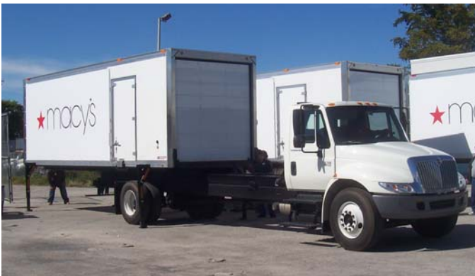
Caption: At the regional market, a body is mounted by a straight-truck power unit prior to making deliveries.
