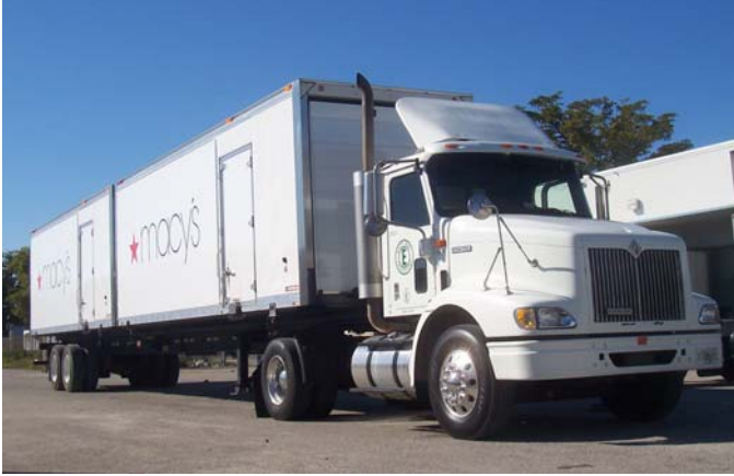
Caption: Two straight-truck bodies being transported on a semi-trailer from Miami to the Tampa or Orlando market.
