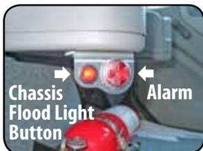
6. The chassis lift lock alarm inside the cab will continue to sound after the truck is turned off. **If the truck is to be parked for an extended period of time, lock the chassis lift hooks.**
