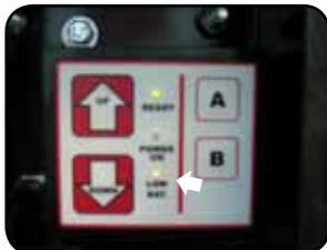
5. If the truck battery is running low, the controller may go into a "LOW BATTERY" state.
