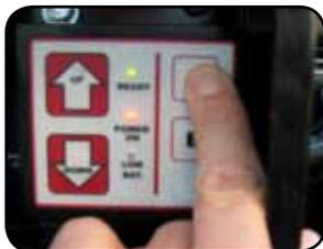
1. Enable the controller by entering the security code. Press the keys in the following order: **A, B, A, B**.
