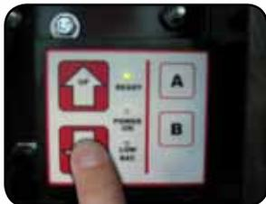
3. Operate the chassis lift by pressing the "UP" or "DOWN" button as necessary.
